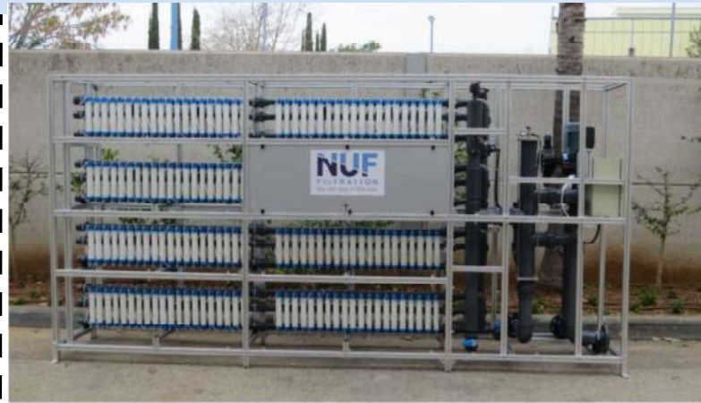
Industrial NUFilter plants – modular, fully automated units for public swimming pools
